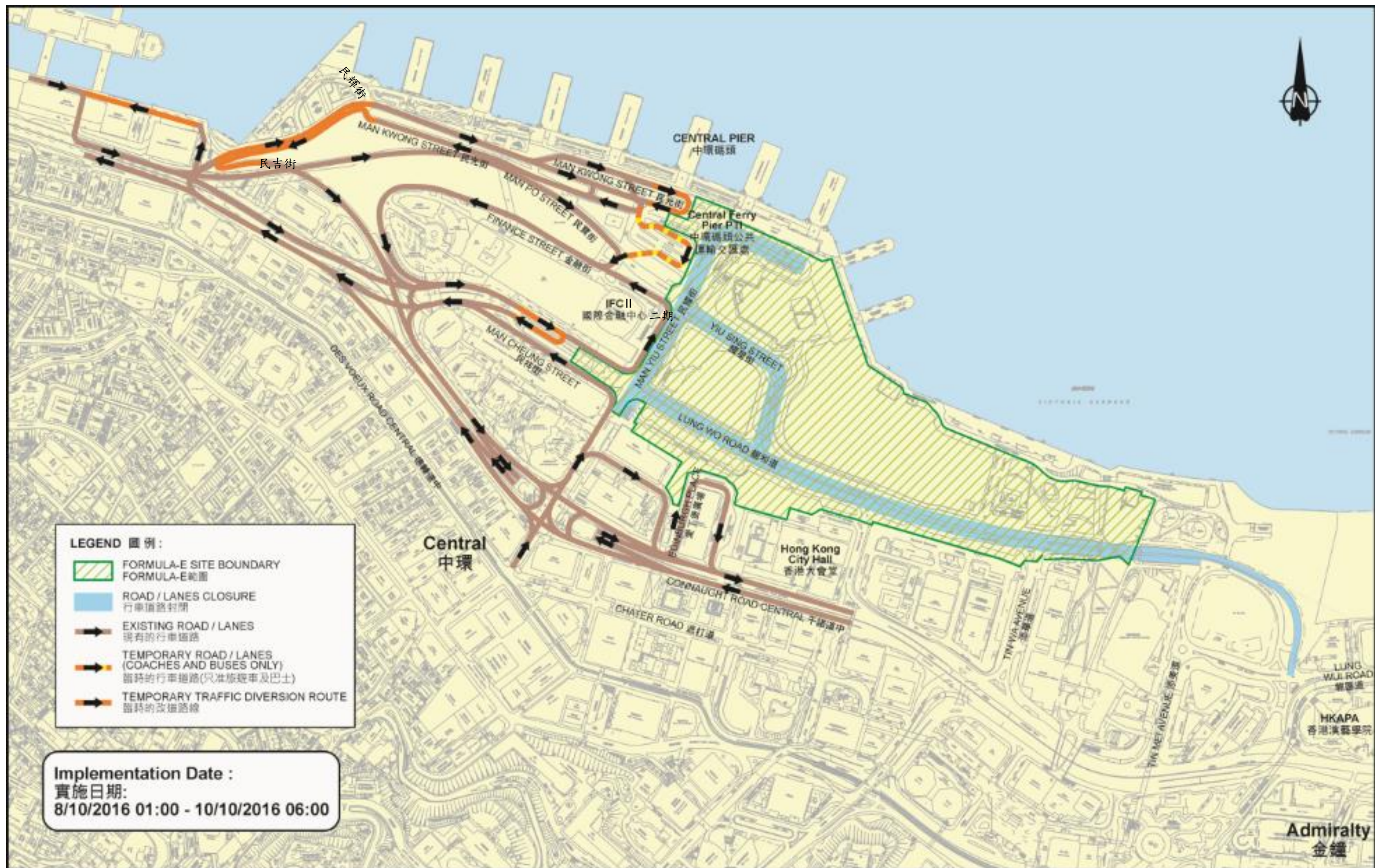
FIG3.2 TEMPORARY TRAFFIC DIVERSION ROUTINGS DURING RACE EVENT (ON THE WEST OF EVENT SITE AREA)
